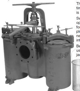
The Plug Type Duplex Strainer is a simple, economical, and trouble free design ... time tested in applications around the world over many years. This type of strainer is actually a high quality, pressure rated plug valve with integral straining baskets.
