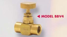
Brass, 1/4" NPT female connections only. Suitable for 600 psi at 300° F maximum; for water, oil or gas service.
