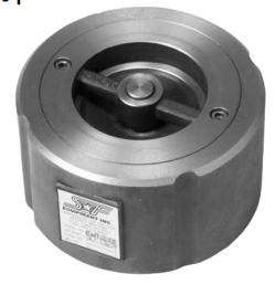
Sure Flow Wafer Check Valves are designed to close before the pump stops completely. This prevents flow reversal which eliminates water hammer and system surges associated with valve closure.
